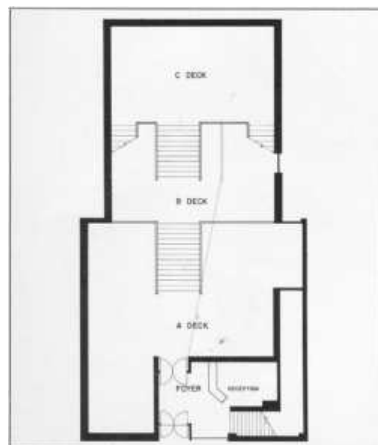
Govett-Brewster Art Gallery, floor plan showing sightline from Foyer doorway to front edge of staircase (A to B deck), and its projection to B deck. Sightline determines new width of staircase (B to C deck).
